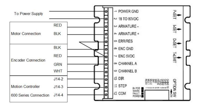
710 Series Wiring Diagram
